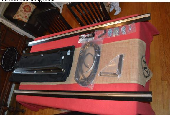
2. Put the frame together since you will be using this for a reference in a short while. The two sides are the longer sections with tracks and then you have a front and back. The front has a rectangle hole for the securement when it is closed. This is different from the rear, which has no hole. The four 90 degree brackets are what will connect it all together. These brackets will be on the inside roof surface, bolting to the frame that will be on the outside during final install.
