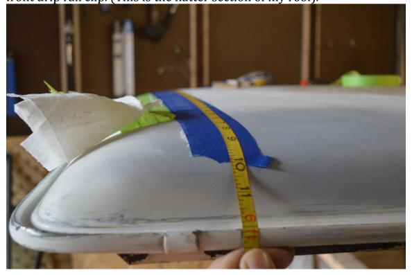
4. What I found easiest since I was by myself for the install, I marked my measurements on the drip rails on both sides (driver and passenger) and ran a "pop string" from one side to the other and popped my line for the front and repeated for the back line.
