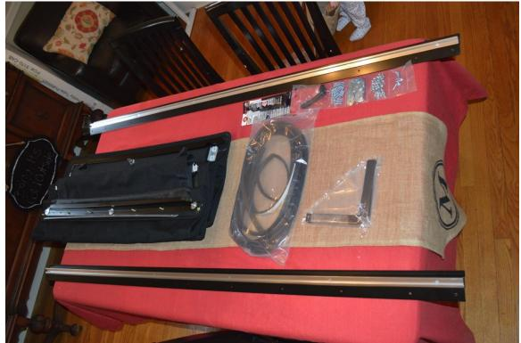
2. Put the frame together since you will be using this for a reference in a short while. The two sides are the longer sections with tracks and then you have a front and back. The front has a rectangle hole for the latching the top when it is closed. This is different from the rear, which has no hole. The four 90 degree brackets are what will connect it all together. These brackets will be on the inside roof surface, bolting to the frame that will be on the outside during final install.
